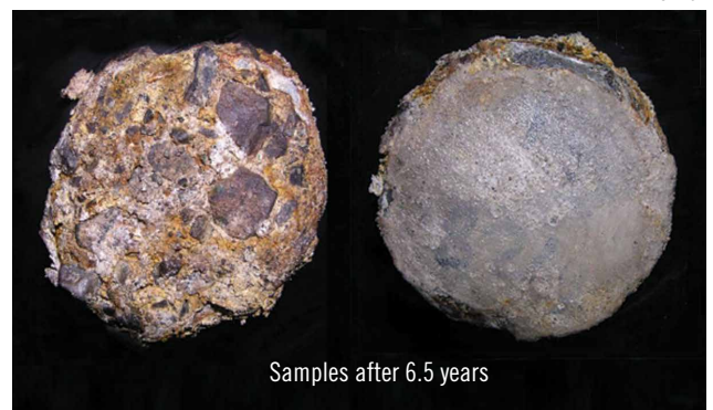
UNTREATED CONCRETE BIO-SAN C500 TREATED CONCRETE
